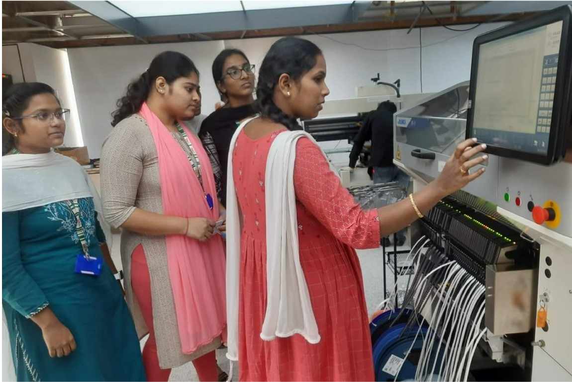
PCB Components Automatic Pick and Place Machine
